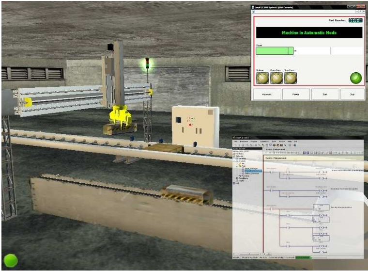
Machines Simulator working, showing the HMI System and EasyPLC Editor in debug mode
